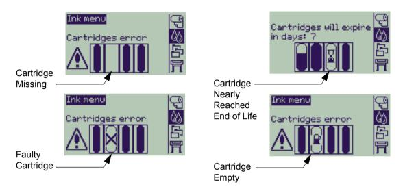
NOTE: If a cartridge has actually passed its expiry date, it will be shown as a faulty cartridge and will have to be replaced.
