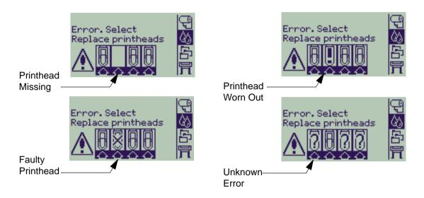
NOTE: An unknown error is displayed when one of the printheads is causing a problem but the system cannot detect which one it is. Refer to <u>Unknown Printhead Error</u> to solve this problem.
