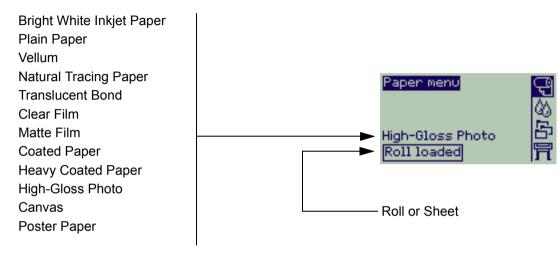
If there is no paper loaded the front panel display shows the following message and you will need to load roll or sheet media.
