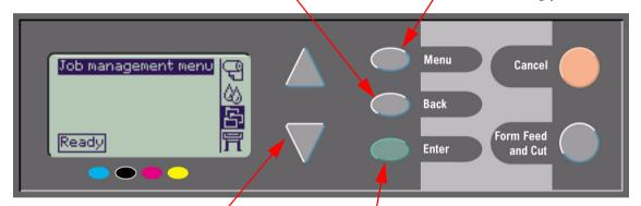
Press the **Up** and **Down** keys to scroll up and down though the menus or menu options.
