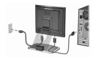
Connecting the VGA Signal and Power Cable
