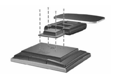
2. Mount the monitor to a swing arm or other mounting fixture by following the instructions included with the mounting fixture to be used.
