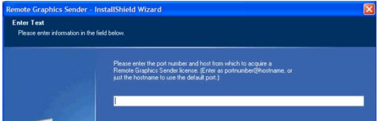
Figure 5-9 Dialog to enter the license server hostname and, optionally, the port number
