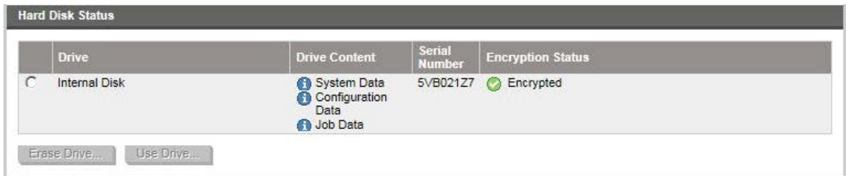
Figure 7: Shows the Hard Disk Status a green check means an encrypted disk is Installed and Encrypted.
