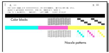
Check the color blocks and nozzle patterns for streaking or white lines.
