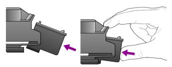
The tri-color print cartridge goes on the left and the black cartridge goes on the right.
