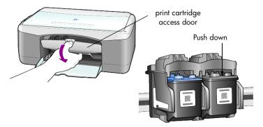
2 After the carriage stops moving, push down on the print cartridge to release it, and then toward you out of its slot.
