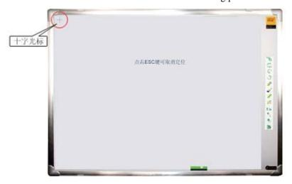
Align the nib of the electronic pen to the center position of cross cursor on the positioning interface and click it, and then finish the positioning after click 7 cross cursors occurred in proper sequence.
