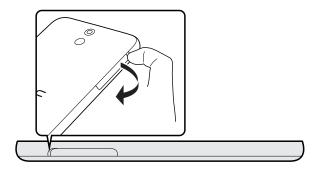
2. With HTC Desire 610 facing down, make sure that the card's gold contacts are facing up and its cut-off corner facing in.
