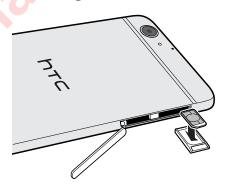
5. When reinserting the tray, make sure it is facing up so that the nano SIM card doesn't fall out. Slide the tray all the way into the slot.
