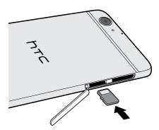
3. To close the slot cover, slide the plastic hinge into the side and press the cover until it clicks into place.
