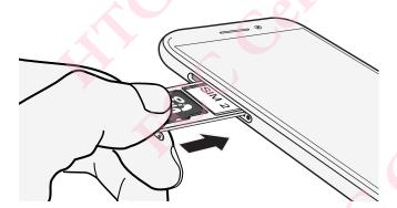
**6.** Make sure the tray is fully inserted and doesn't protrude from the slot.
