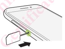
When inserting the eject tool into the tray eject hole to remove the card tray, do not obstruct the tray to avoid damaging the eject mechanism inside the slot.
