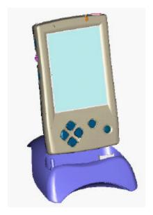
If the battery gets very low, your Bluebird displays a warning message. If this occurs, save any unsaved data you are working on, perform a synchronization with your computer, then turn off your Bluebird If your Bluebird does shut down, you still have about 40 hours to recharge the battery before you lose the data on your Bluebird.
