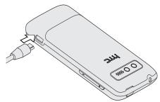
3. Plug in the power adapter to an electrical outlet to start charging the battery.
