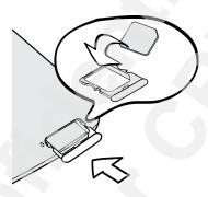
3. Insert the SIM card tray into its slot.
