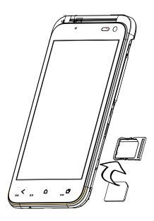
3. Slide the SIM card tray into its slot.
