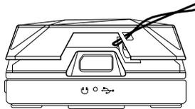
3. Attach the loop over the small hook at the bottom of the back side of the phone.
