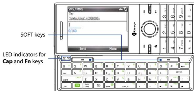
The LED indicators corresponding to the **Cap** and **Fn** keys on the keyboard display solid orange color when the **FN** and **SHIFT CAPS** keys are pressed to turn on their functionality. Press a desired corresponding key and turn them off after use.
