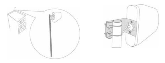
■ Installation of YAGI antenna as donor antenna
