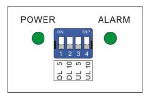
Switches 1.2 represent Downlink and 3.4 represent Uplink. When it is necessary to adjust the gain by DIP switch, firstly please adjust Downlink gain according to input signals, secondly please adjust Uplink gain according to Downlink gain.
