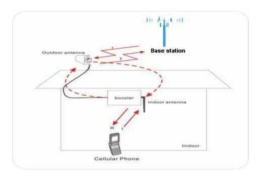
If isolation can't be achieved by the limited distance, the roof of the building or any other barriers can be used in between to increase isolation.
