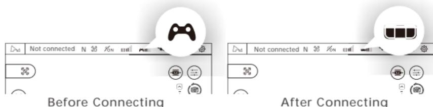
(4) Start binding (This step is only required when first binding or replacing the transmitter, you need to do it manually.)
