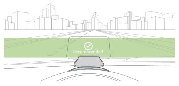
Before removing the protective sheet from the base, open the lens and try looking through it. Make sure it doesn't block your view — it should be at the bottom of your line of sight.
