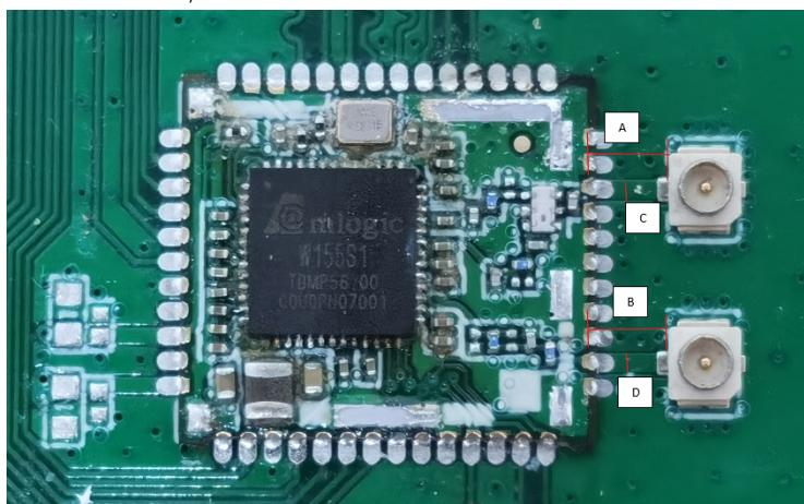
Circuit between the connector to module distance: 4mm
