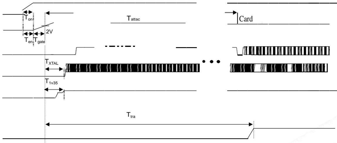
**T<sub>on</sub>**: The main power ramp up duration
