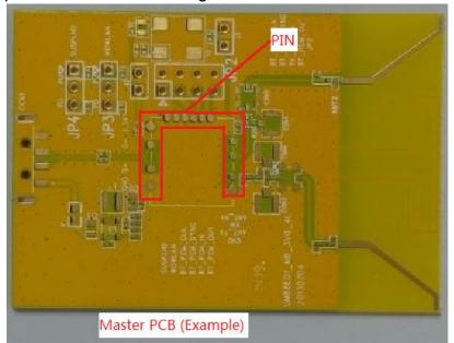
3. Place the Module on the Master PCB. Then solder it in sequence : 1.2.3
