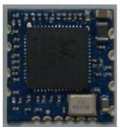
2. Ready the Master PCB which will connect with RTL8723BU Module. Check connection pads is clean for soldering.
