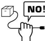
Pull out the power cord with holding the plug, not the cord.
