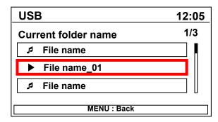
Press the [Tune(Up)], [Tune(Down)] keys to search for the desired file and press the [OK] key to select.
