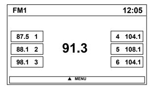
After selecting frequency ▶ Press and hold the desired preset button from [1] ~ [6].
