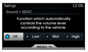
The volume level is controlled automatically according to the vehicle speed.
