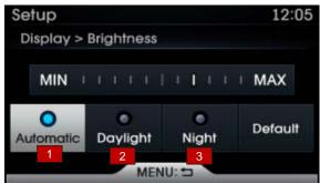
Use [HD/CAT(Left)], [Folder(Right)] to adjust the screen brightness or set the Brightness on Automatic, Daylight, or Night mode.
