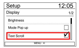
This feature is used to scroll text displayed on the screen when it is too long to be displayed at once.
