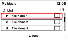
Use [Tune(Up)], [Tune(Down)] and the [OK] key to search and select files you want to delete and press the [Delete] button from the Menu.
