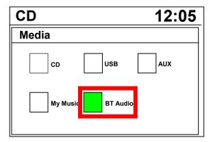
If the Bluetooth® device is not connected, then the [BT Audio] button will be disabled.
