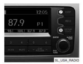
Press 6 button more than 0.8 seconds or longer to save the current station to the respective button with a beep.
