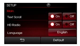
3. Press the [On] or [Off] button next to the Text Scroll menu to turn the feature on or off.
