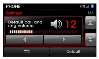
3. Use the [left] / [right] buttons to control the volume to the desired level.
