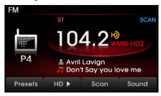
**HD Radio** is a digital radio technology used by AM and FM radio stations to transmit audio and data via a digital signal in conjunction with their analog signals.
