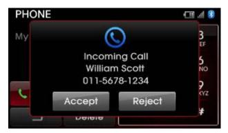
2. Press the [Accept] button or the [Call] key on the steering wheel controller to take the second incoming call. Press the [Reject] button to reject the second incoming call.
