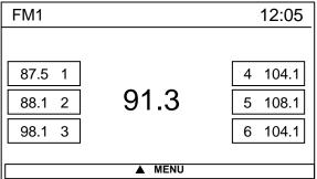
The 6 preset buttons are displayed. Press the [1]  $\sim$  [6] keys to play the desired preset.
