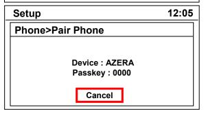
From your mobile phone, search for the car audio system. The initial passkey is "0000". Once pairing is complete, the following screen is displayed.
