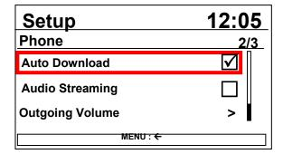
This feature is used to automatically download mobile phone contacts once a Bluetooth phone is connected.
