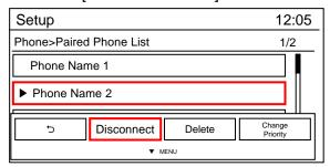
From the paired phone list, select the currently connected device and press the [Disconnect] button from the Menu.
