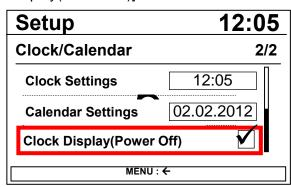
When turned on, this feature is used to display a clock on the screen when the audio system is turned off.
