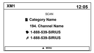
Press the [SCAN] key to scan all channels with superior reception for 5 seconds each.
