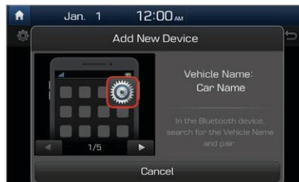
3 Ensure that the Bluetooth passkeys displayed on the Bluetooth device screen and the system screen are the same and confirm the connection from the device.
