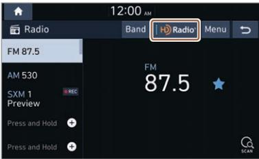
In the HD mode, HD Radio station buttons are displayed at the top of the radio screen. Press a button to select one of the available HD Radio stations.
