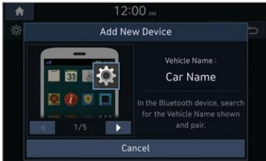
4 Ensure that the Bluetooth passkeys displayed on the Bluetooth device screen and the system screen are the same and confirm the connection from the device.
