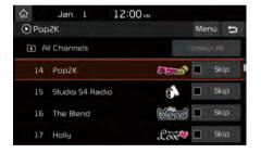
Select the desired category and the channel. Once selected, the previous screen will be restored and the selected channel will begin playing. If you select the skip button, you can scan channels using the seek TRACK key or the TUNE knob by skipping the channels that you chose to skip.
