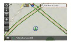
You can use this menu when the vehicle shift lever is in P (Park) and there is no destination set. Press the Search lcon(Place or Address) to move to "Places".
