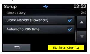
This feature is used to set time automatically by synchronizing with RDS.
