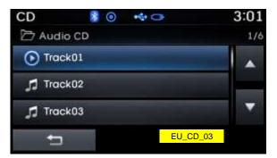
Turn the [TUNE/FILE] knob left/right to search for tracks. Once the desired track is displayed, press the knob to select and play.
