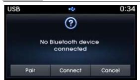
• If Bluetooth® devices are paired but none are currently connected, pressing the [PHONE] key or the [3] key on the steering remote controller displays the following screen. Press the [Pair] button to pair a new device or press the [Connect] to connect a previously pair device.
