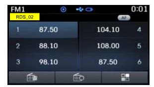
While listening to a frequency you want to save as a preset, press and hold one of the [1] ~ [6] preset buttons (over 0.8 seconds) to save the current frequency to the selected preset.
