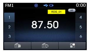
Press the [Preset] button to display the broadcast information for the frequency saved to each button.
