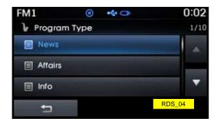
Turn the [TUNE/FILE] knob left/right to search for the desired program type. Once you find the desired program type, press the [TUNE/FILE] knob.
