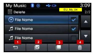
Press the [Mark All] button or individually select the files you want to delete. Once files are selected, the [Unmark All] and [Delete] buttons will be enabled.
