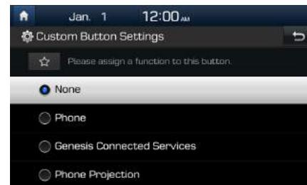
Setting it to a feature that you frequently use will allow you to access the feature quickly and conveniently anytime. For example, setting it to **My Menu** will enable you to access the My Menu screen by pressing the **☆** key.
