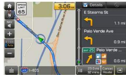
Additional info of Freeway exit or Rest area can be displayed by selecting the
