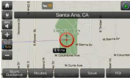
While the destination is set, the buttons **Start Guidance**, **Routes**, and **Add Waypoint** appear. Select the desired button to change a destination or add a waypoint.
