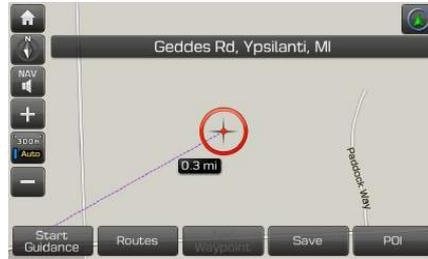
Touch the compass arrow icon to toggle between a map oriented to the North, oriented parallel to the vehicle’s heading and 3D View.
