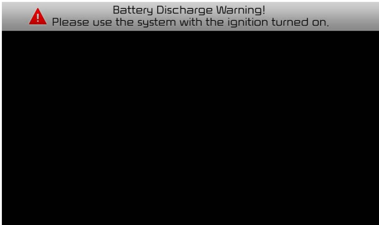
Use the system only when the engine is running. If the system is turned on with the engine off, then the following warning will be displayed.
