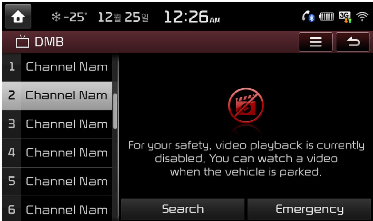
When use video mode such as DMB, DVD an VCD while driving, the display will turn off for the safety and the message related to driving regulations will be shown up. Although the display off, sound will play. If gear changed to P, or parking brake on, the display will turn on again automatically.
