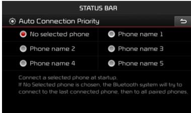
When ignition on, connect to the Bluetooth device automatically. If connection to the selected device failed, it will connect previous connected device. If also failed to connect to the previous device, it will connect to registered devices automatically.
