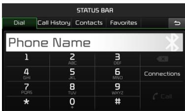
1. Keypad: Input numbers you want to call. After input speed number and then long press the last digit, you can call the number saved in the mobile phone as speed dial.
