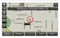
Touch the compass arrow icon to toggle between a map oriented to the North, oriented parallel to the vehicle's heading and 3D View.
