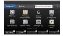
On the button where locations are not registered, the  $\oplus$  icon is displayed. When a location is registered, the  $\oplus$  button disappears and the buttons 1 to 3 are displayed as your favorite places.
