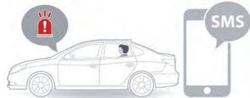
When the driver's door and a rear-seat door are open before turning on the vehicle but only the driver's door is open after the vehicle is turned off, the instrument cluster alerts the driver with a message and sound to check the rear-seat.
