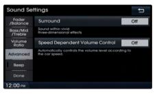
This is used to set the Variable-EQ (or Surround) and Speed Dependent Volume Control features.
