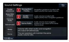
These options are used to set the volume ratio by selecting from Navigation Priority/ Audio Priority/Same Ratio.
