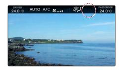
When DUAL is disabled, the driver-side and passenger-side temperatures are controlled simultaneously.
