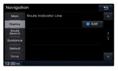
This menu is used to set the color of the Route Indicator line displayed when receiving route guidance.
