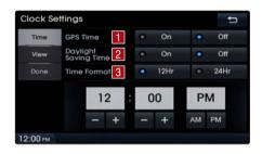
This menu is used to set the time used within the Navigation system.
