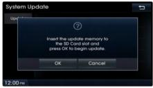
After inserting the SD card with the update file, press **OK** to start the update.
