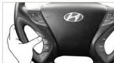
1. Press the **VA** key on the steering wheel remote controller.
