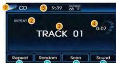
1. Mode display : displays that the current mode is CD mode.
