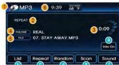
1. Mode display : displays that the current mode is MP3 disc mode. (MP3 files on DVD discs are not supported.)
