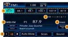
1. Preset Button: desired HD frequencies are saved for convenient frequency selection. Saves up to HD1~HD8 according to sub broadcasts.
