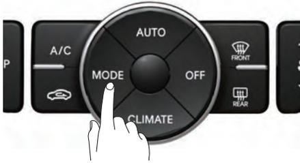
1. Press the **MODE** key. The fan direction will be changed.
