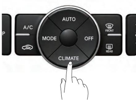
1. Press the **CLIMATE** key to display the HVAC system status on the entire screen.
