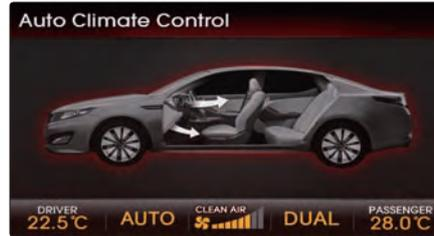
2. When in the AV, Navigation, or Bluetooth® handsfree mode screen, press a HVAC key, such as **TEMP**, **AUTO**, or **A/C** to display the HVAC system status bar at the top of screen.
