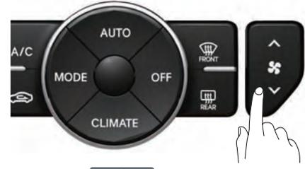
1. Press the **fan level** key. The fan level will be changed.
