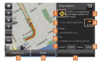
Select the traffic information on the traffic list to display the detailed screen as shown in the screen.
