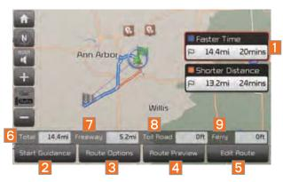
When the alternative routes option is enabled in navigation setting, two routing options are displayed based on faster time and shorter distance.
