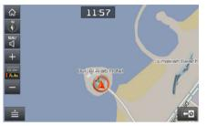
Press the **N** button to set the "2D heading up" mode. The map will rotate automatically when your driving direction changes.
