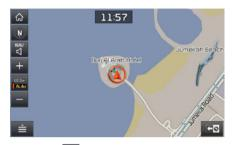
Press the velocity button to set the map orientation to "2D north up" mode. The upper side of the map will point to the north no matter what direction you travel.
