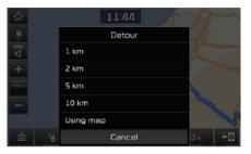
You can set the detour option from this screen. Press the Using map button to set the detour points using the map view.
