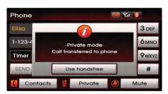
Mute: Use this function to mute the outgoing volume. Pressing the Mute button will display the at the top right side of the screen and the caller will not be able to hear the conversation taking place in the car. Press the Mute button again to release the Mute function.
