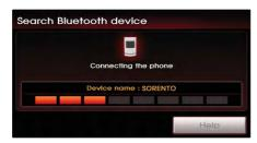
(5) When pairing the car handsfree from the mobile phone, a passkey input window will become displayed on the mobile phone screen. Input the passkey set within the car system into the mobile phone input window. (The factory state passkey is 0000.) As shown in the figure, once the passkey becomes successfully inputted, the Bluetooth connection between the car system and mobile phone will start.
