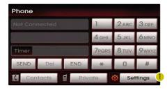
Settings: The user can set environment settings for the Bluetooth handsfree, such as pair/delete mobile phone, connect/ disconnect mobile phone, set call volume, change device name and change passkey. ■ When a mobile phone is connected
