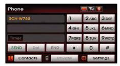
The Press and hold (over 0.8 second) the SEND button on the PHONE screen or the key on the steering wheel.
