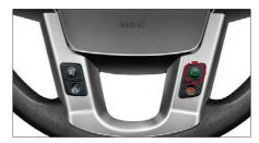
① While in AV mode or Navigation mode, press the PHONE key or the key on the steering wheel.
