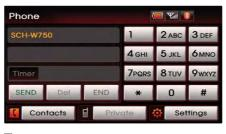
2 To reject the incoming call, press the Reject button or the key on the steering wheel. The incoming call will be rejected.
