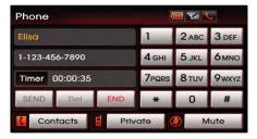
If you wish to switch the call to the mobile phone while talking on the car handsfree, press the Private button or press and hold (over 0.8 second) the key on the steering wheel.
