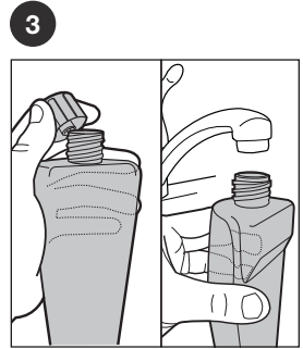
Turn Cap counterclockwise to remove. Fill tank with water.
