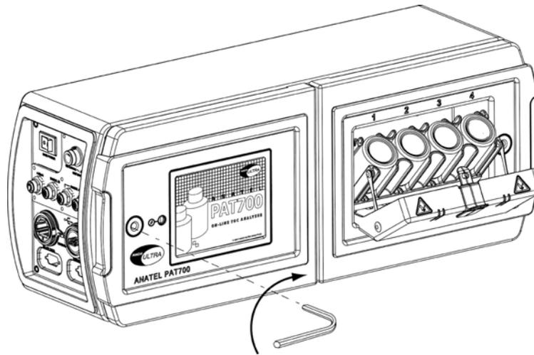
Figure 2-7 Using Allen wrench to access wiring connections
