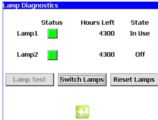
Figure 8-2 Lamp test dialog box
