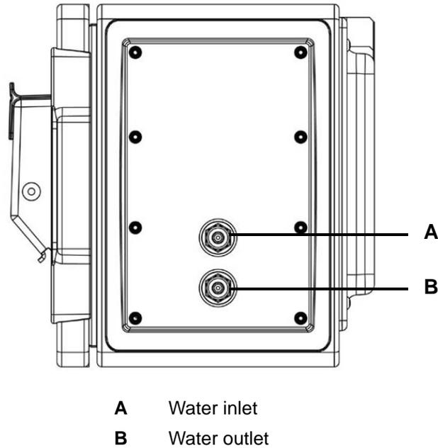
Figure 2-6 PAT700 water inlet and outlet connections
