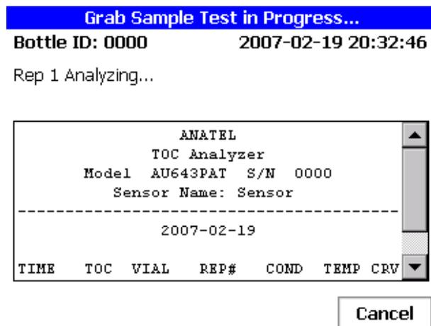
Figure 6-17 Grab sample test in progress dialog box
