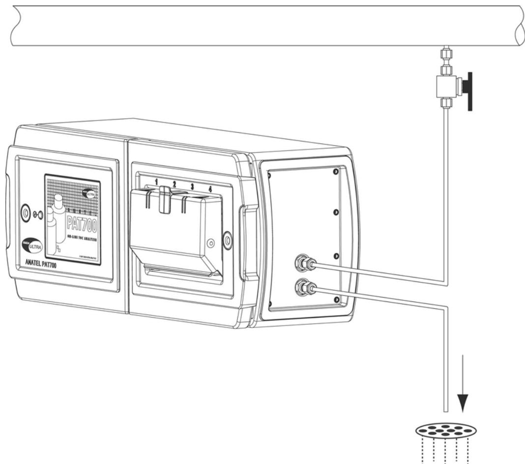
Figure 2-5 PAT700 connection to isolation valve
