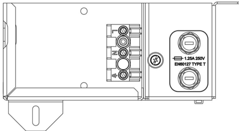
Figure 2-9 PAT700 power supply wiring terminals
