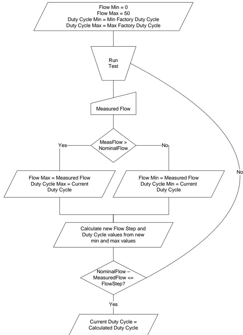
Figure 8-16 Pump calibration flow diagram
