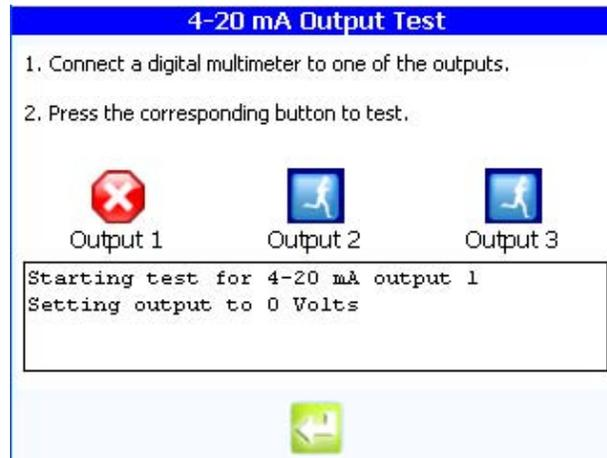
Figure 8-12 4-20 mA output test dialog box
