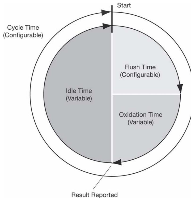
Figure 4-1 The TOC analysis cycle
