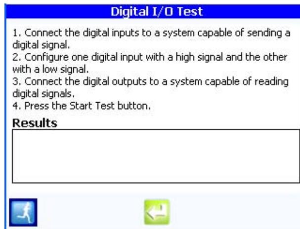
Figure 8-11 Digital I/O test dialog box
