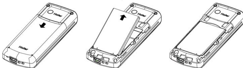
Installing the battery
