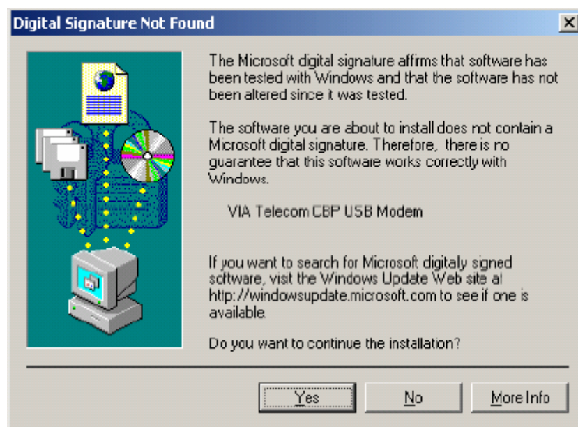
Figure 11 – Windows Device Manager’s Device-Discovery Notification that the CBP USB Modem Device- Driver Lacks WHQL Certification
