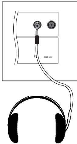
Plug a set of headphones into the 3.5mm mini-jack socket on the rear panel of the set.
