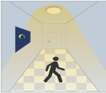
When motion detected, insufficient daylight, light ON.
