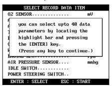
b ULTRASCAN plus will show you the whole live data parameters available in the control system you selected. Locate the highlight bar on the desired parameter and press the [ENTER] key.
