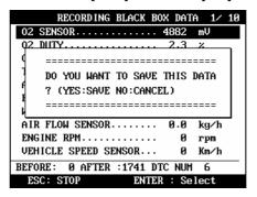
b When pressed [YES], a dialog box follows and asks you to input the test date. Enter the date and press the [ENTER] key to save the recorded data to ULTRASCAN plus memory.
