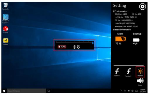
LCD brightness based on the ambient light.
