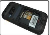
4. Insert the battery back to the compartment while ensuring gold contacts align with the device contacts. Then move the slider to the left to secure the battery.
