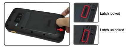
2. Insert a small flat head screwdriver into the notch and gently pry up the cover.
