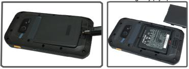
3. Remove the battery, if inserted. The battery is secured by a red slider. Move the slider to the right so that you can remove the battery.
